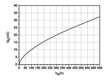
Fig.3-Capacitance vs. Reverse Voltage
